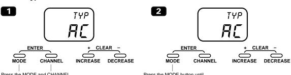
Press the MODE and CHANNEL buttons simultaneously and hold while turning on the transmitter. Press the MODE button until TYP appears on the screen.
