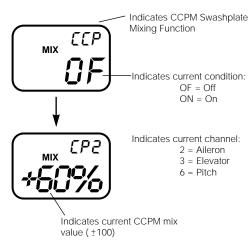
Please refer to the helicopter manufacturer's instructions for proper mixing values. Please also note that if control system interaction exists (pitch to aileron, pitch to elevator movement, etc.), it will be necessary to alter the travel adjust values for channels 2, 3, and 6 to correct this situation. Please refer to page 74 of this manual for further information.
