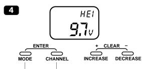
Press the MODE and CHANNEL buttons simultaneously until a beep is heard.
