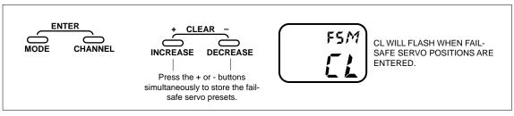
1. Press the MODE button until FSM appears on the screen.
