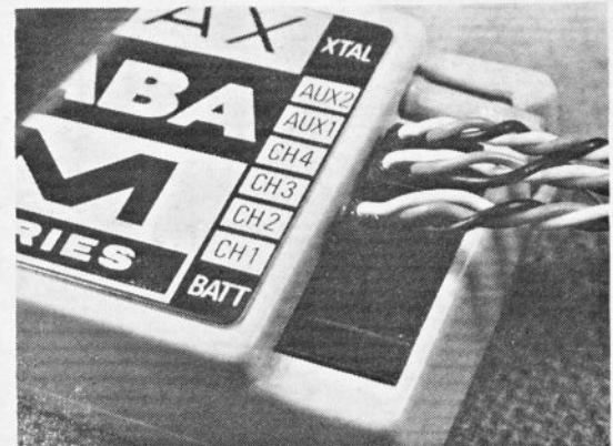
The single deck receiver is very compactly laid out. Note positioning of the plug-in crystal and servo plugs, which have the wires moulded-in for safe handling.
