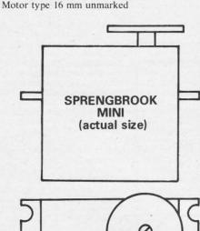
Weight: 45 gms. Output devices: Disc 3 lengths of arm. Reverse rotation model: Label identification.
