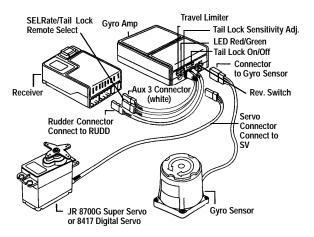
Step 3: On the amplifier, locate the SV (Servo) receptacle. Plug the rudder servo into this receptacle, noting the correct polarity as indicated by the shape of the plug, as well as the wire color.
