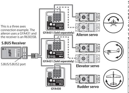
S.BUS connectivity minimizes wiring. The GYA430 and GYA431 can be connected by one 3-way hub. The aileron, elevator, and rudder servos are output from the gyro. Standards servos can also be used. When an R6303SB is used the CH switching mode is set to group 7. The normal group 7 CH outputs are CH3, CH11, and CH12. CH3 is the throttle channel and CH11/CH12 are spare channels.
