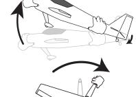
Tilt the airplane to the left on the ground and check that the rudder operate to the right. (In the case of rudder control)
