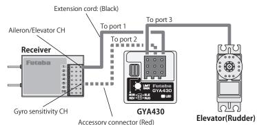
Gyro gain CH(Receiver)←connect→Port2(GYA430)
