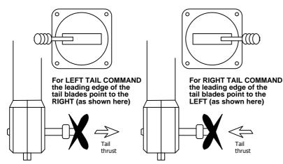
If the tail blades move in the wrong direction change the servo reversing of the tail rotor channel in your transmitter and recheck the movement of the tail blades.
