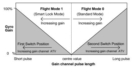
The Gyro gain channel acts as both gyro mode switch and gain control
