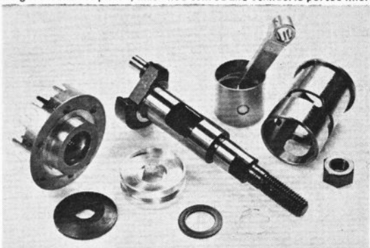
Included with each O.S. Max 25F-SR is the effective OS-762 silencer, specially designed for this engine. Below: Some Max 25F-SR parts, showing bowl-and-squish cylinder head, large diameter shaft, lightweight Meehanite piston, machined conrod and Schnuerle ported liner.
