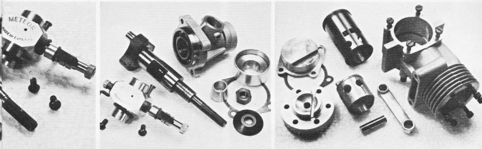
Below and below right: 1976 Meteor 60 parts. New castings are produced by gravity die casting process. Cylinder-head now has squish-band. Carburettor is of two-needle type with airbleed.
