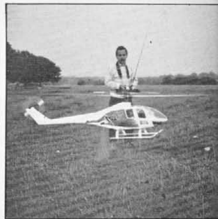
A Robbe Avantgarde belonging to Jim's flying buddy, John Sowersby. This model also has an OPS pipe but this time it's fed by a Super Tigre .61, also a successful marriage. One of the nice things about the OPS pipe is that all the 'crud' is blown down and away from the model, a much more refined way of doing things.
