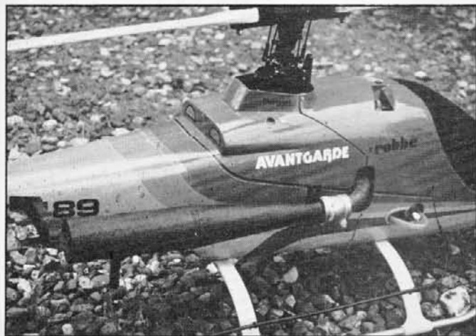
A Robbe Avantgarde belonging to Jim's flying buddy, John Sowersby. This model also has an OPS pipe but this time it's fed by a Super Tigre .61, also a successful marriage. One of the nice things about the OPS pipe is that all the 'crud' is blown down and away from the model, a much more refined way of doing things.
