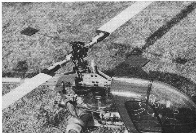
Left: complex and highly efficient rotor head of the Ishimasa Playboy Collective. Right: state-of-the-art Kait Baron 20 - see text.
