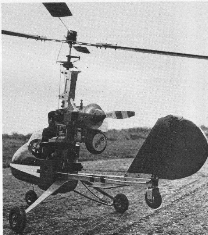
Above and left: two views of John's autogiro which appears on close inspection to have more modifications than he mentions in the text — an extra wheel at the tail for one! His spin-up device, mentioned briefly in the text, can be seen to the rear of, and below, the spinner.
