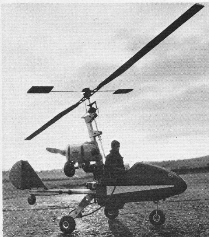
Above and left: two views of John's autogiro which appears on close inspection to have more modifications than he mentions in the text — an extra wheel at the tail for one! His spin-up device, mentioned briefly in the text, can be seen to the rear of, and below, the spinner.
