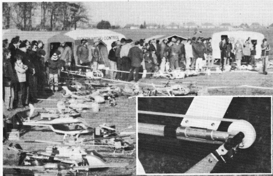
Above: new Morley head also fitted to Jim's own four-blade Puma. Below: Slough Fly-in good assortment of models, even more arrived later. Inset below: this Mick Harris developed single blade rotor has no thrust ball races, counter-balance weight changes pitch with the blade thus there is no outward force on the bearings.
