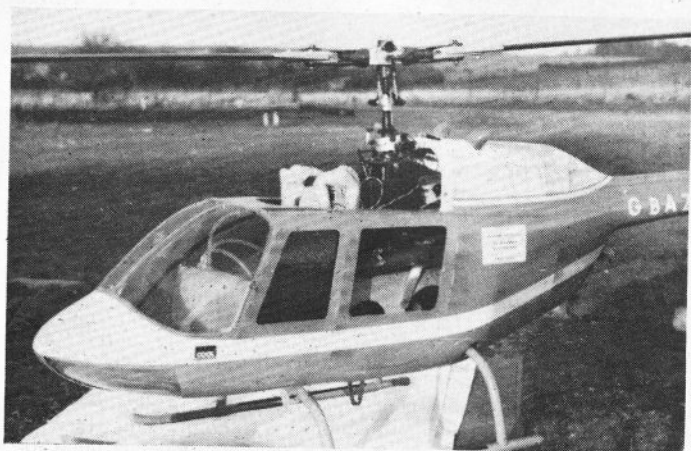
Above: John is very pleased with his latest 'creation' (modelled on a full size Jet Ranger ) which is fitted with his own design 'flybarless' rotor head. This model utilises various parts taken from a selection of model helicopters to 'combine the best of all worlds.'
