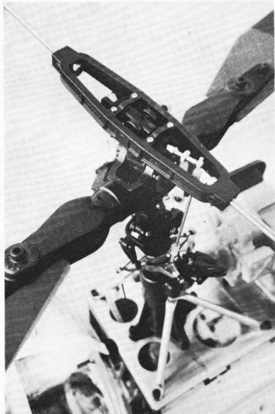
Below; close-up of the Lama rotor-head with connecting links to swash-plate.
