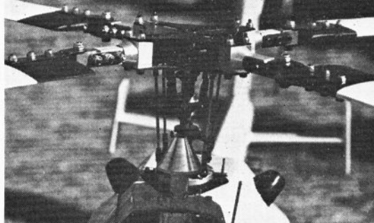
A close-up view of the new Schluter four-blade main rotor, designed for use with Heliboy mechanics. It utilises many of the existing two-blade rotor head parts. Below is a candid shot of Jim Morley's twin-engined Sea King .
