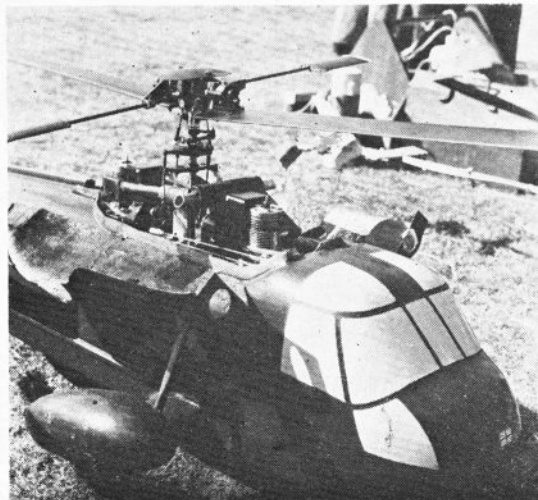
A close-up view of the new Schluter four-blade main rotor, designed for use with Heliboy mechanics. It utilises many of the existing two-blade rotor head parts. Below is a candid shot of Jim Morley's twin-engined Sea King .
