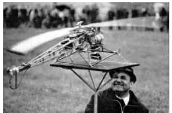
Heinemann Bros.' Test rig for 63 in. dia. Super Tiger 60 powered entry, 1,200 r.p.m., weight 9 lb.
