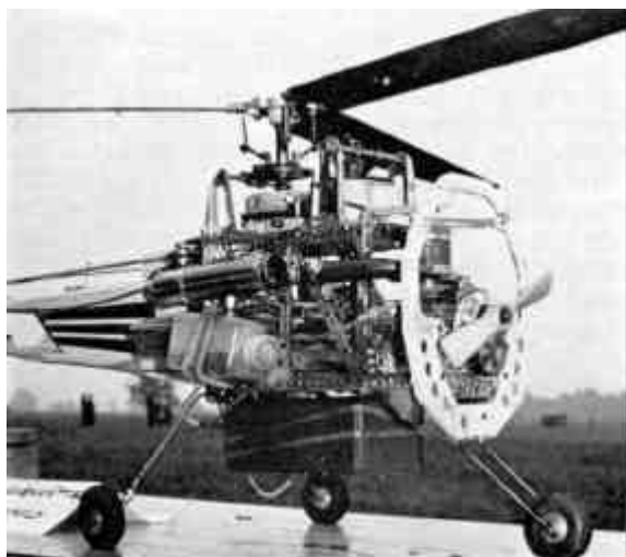
Ing. J. Berkenkotter's tri-bladed 52 in. diameter model is 9 lb.; used Super Tiger G. 60 engine, 700 r.p.m. main rotor. 3,500 r.p.m. tail rotor.
