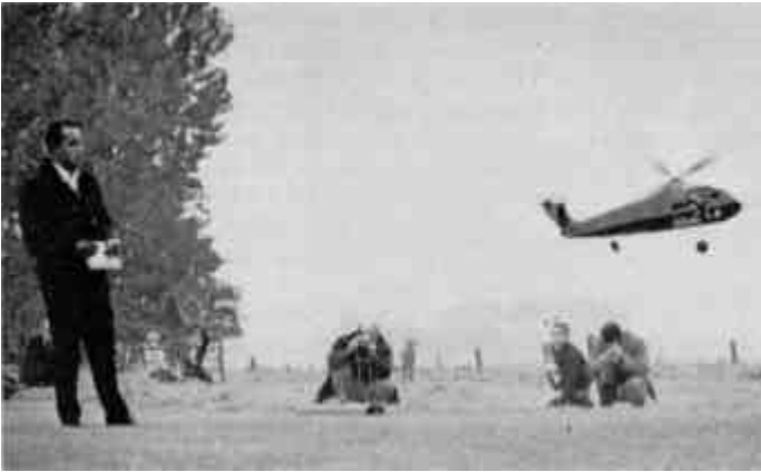
Author's winning entry at 1 st Helicopter International, Harse-Winkel, Germany. Four-blade, main rotor is 47 1/2 in. dia. Super Tiger G60 R.C. engine
