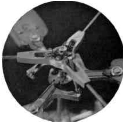
Above left; Power unit on the Plested "Whirl-wind" with central box structure housing R/C and rotor drive. Above right; Gyro bar and rotor hub of "Susie" shows pitch links from bar to blade pitch arms. Below; John Burkam's (U.S.A.) "Super Susie" tri-blade rotor has 32 oz. Thrust, carried four servos. Fuselage is open channel 0.032 in. alum. Gross weight 29 ozs.
