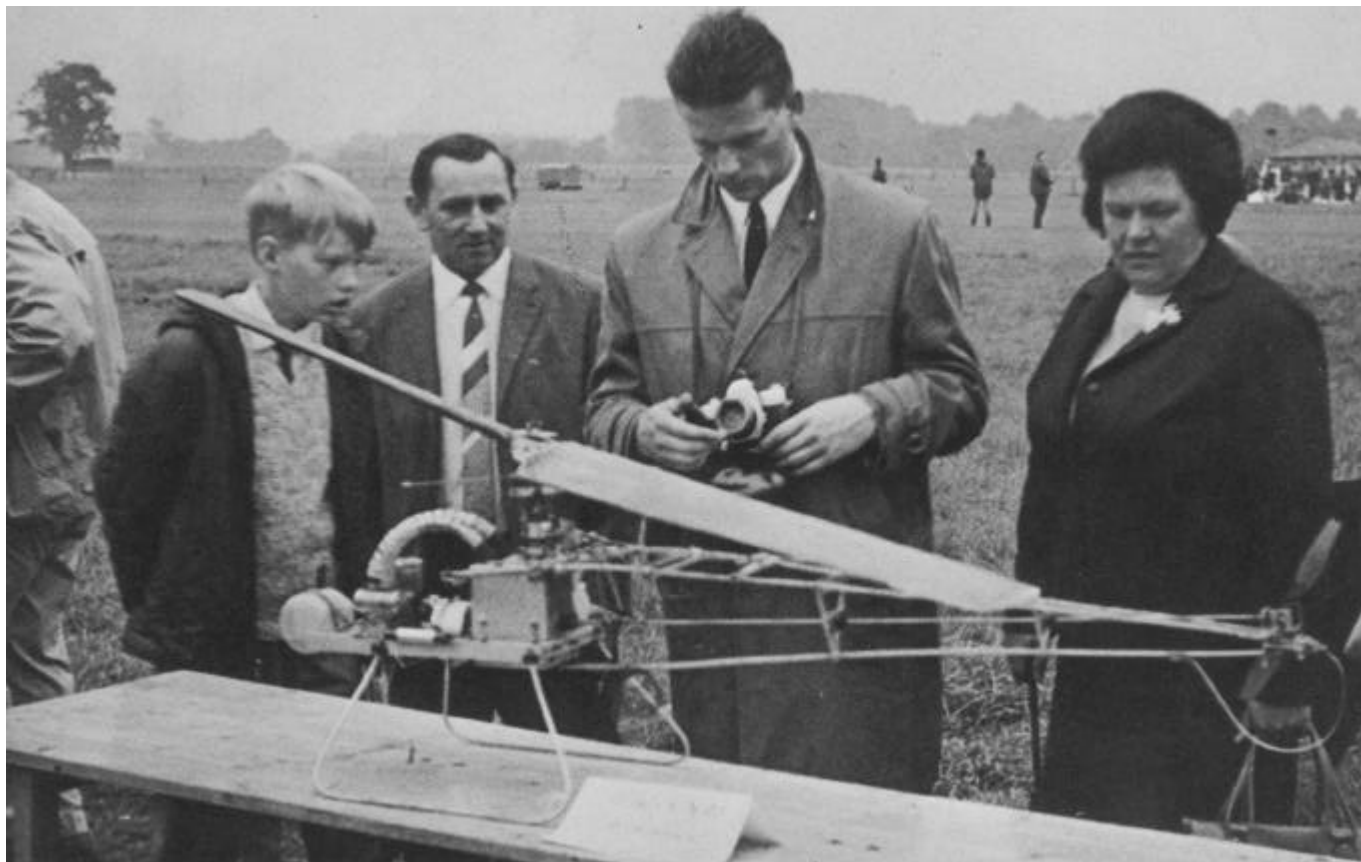
Flexible tubes carried exhaust oil residue back to rotor gearcase. The control system is almost exact replica of Bell 47G. H. W. Knaaf. DNF.
