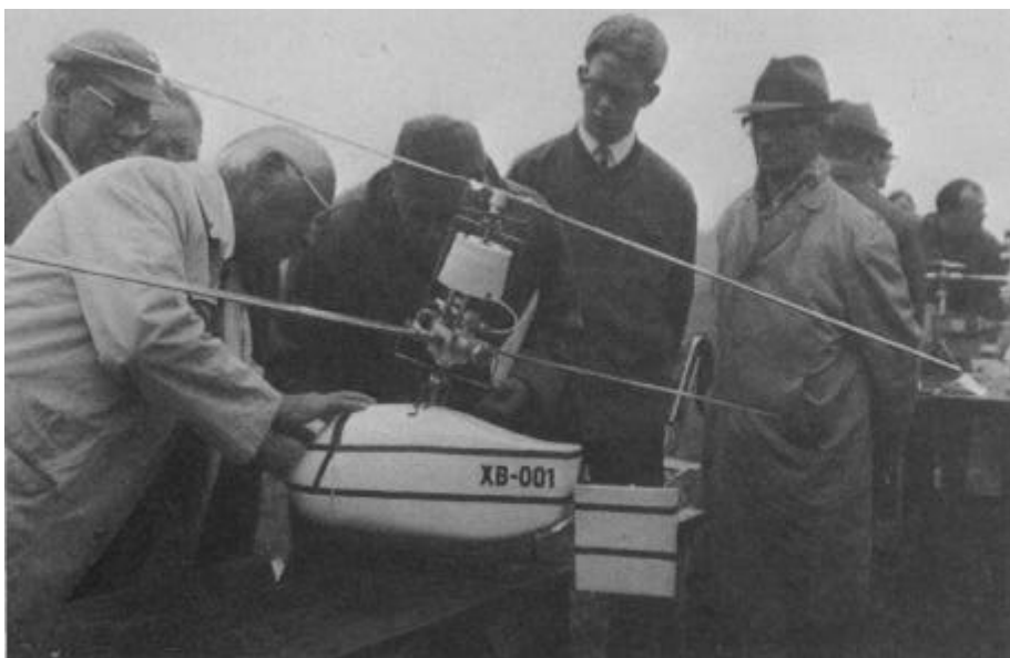
Complete cancellation of torque effect was attained by engineer Stehr from Dortmund, using counterrotating rotors. One engine for each. How would you like to help him start it going?
