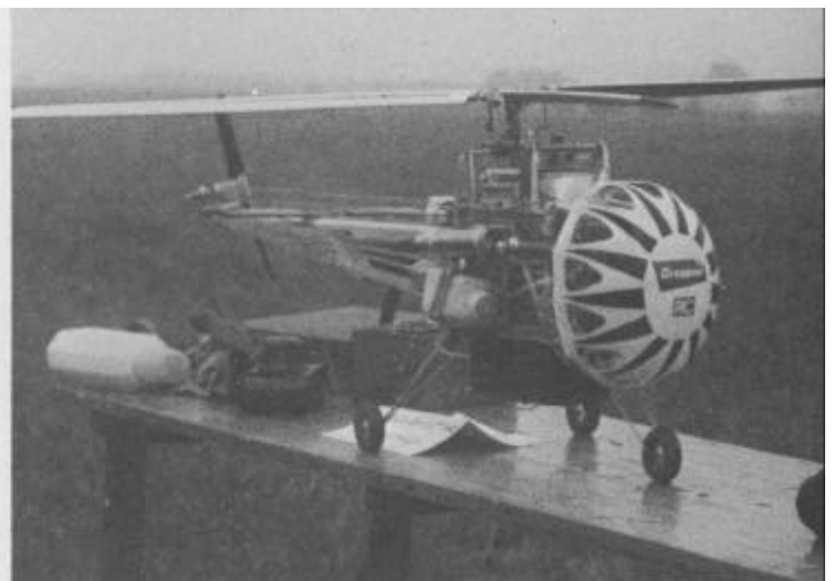
About the most ingenious model entered, Bergenkotter's did not fly. The whole midsection of fuselage was of lattice construction. Complex!
