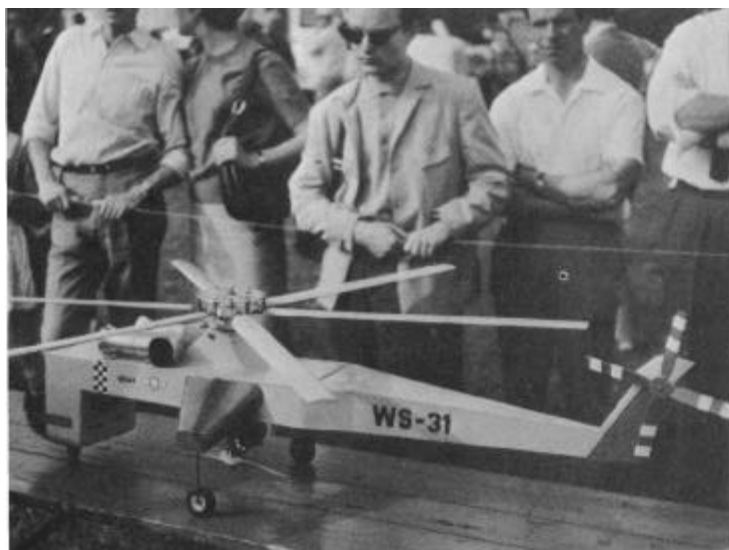
Semi-scale cargo helicopter built by Dr. Schlattmann uses regular prop on underslung engine for torque reaction. Tail rotor apparently dummy.
