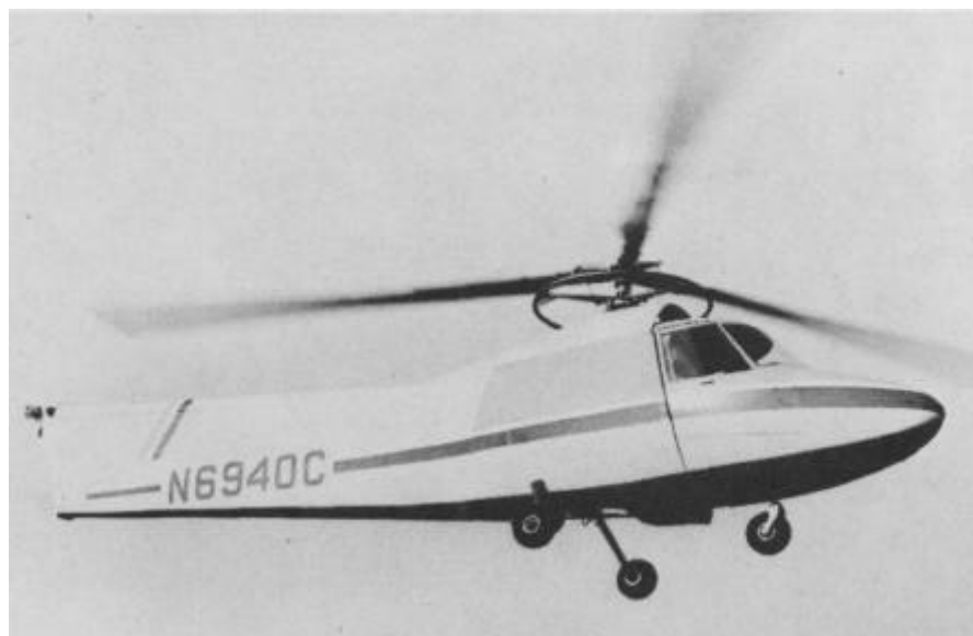
Below: First tests of Lockheed's rigid-rotor helicopter concept were made in a McCoy .60 powered model operated by 8-channel Citizen-Ship reed set.
